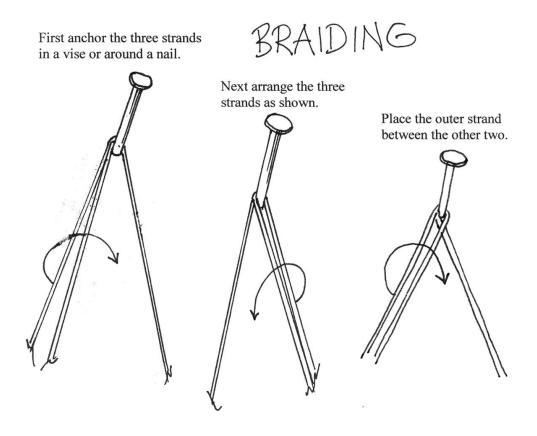
Alternate placing each outer strand between the other two.
